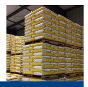
In 2019, Trouw Canada changed its palletizing to be shrink-wrap free, not only reducing plastic usage, but also costs, and eventually reducing the capex cost of new production lines.
